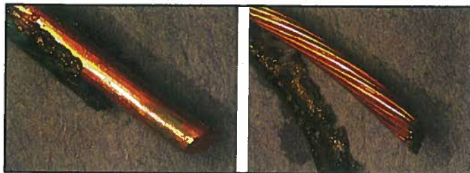
Pictures 12 and 13: Solid and stranded conductors after cleaning in a mix of 3:1 DMSO and MEK at 71 deg C after one hour in an ultrasonic cleaner.
