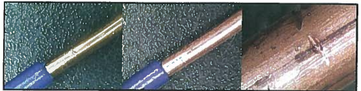
Picture 3, 4, and 5: Freshly stripped wire, etching after "Branson OR" soak, close-up view of "Branson OR" soaked wire.
