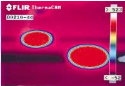
Photo 5—Thermogram of 2 burners on a glass cooktop, showing a lack of heat transfer to other burner locations.
