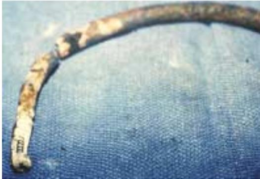
Photo 4—Failed sheath heating element.
