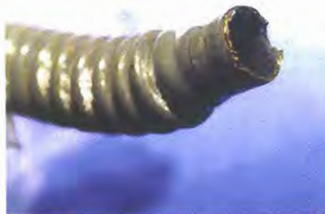
Photo 4. Side view of gal line in Photo 3, with the polymer coating still relatively intact because of protection provided by the brass nut.
