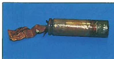
Figure 1. Lithium-Ion 18650 Cell Heat Exposure
