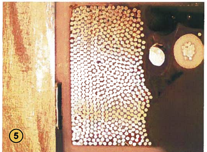
Photo 5 depicts the primary windings after polishing with 600 size grit.
