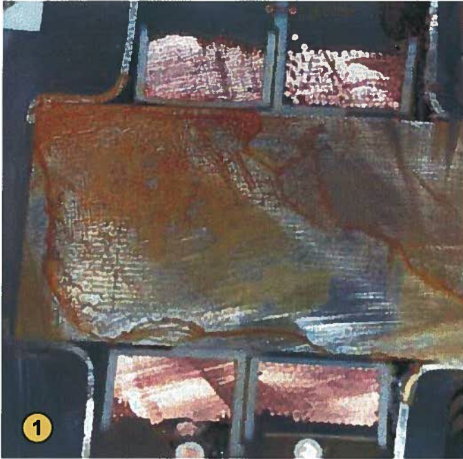
Photo 1 shows a cross section of a transformer after it has been potted and sectioned in half. The primary windings are on the left and the secondary are on the right.
