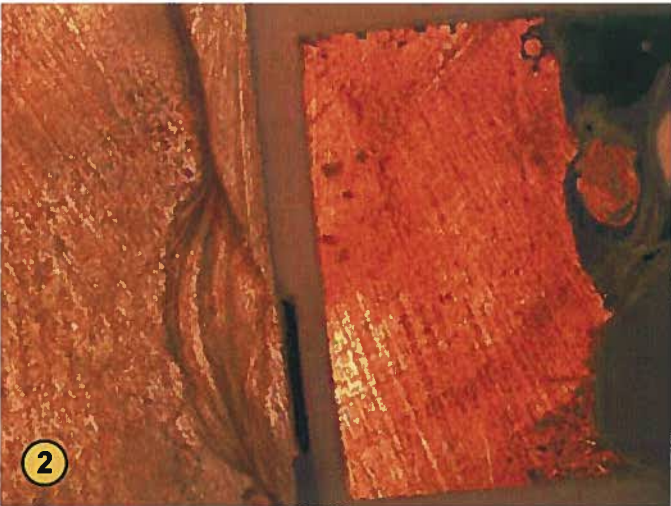
Photo 2 is a microscopic view of the primary windings (the right side of the picture) after sectioning (sawing) but prior to polishing. Notice how the fine conductors are somewhat smeared together by the action of the cutting wheel. The material to the left of the picture is a part of the iron core / laminate stack.
