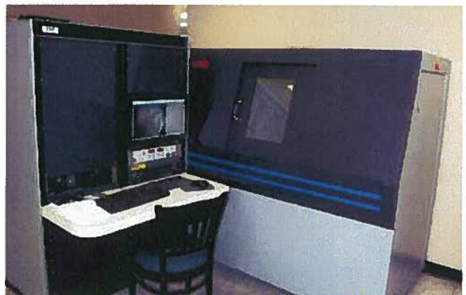
(Photo 2) Larger cabinet with Hamamatsu x-ray source
