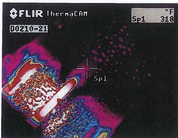
(PHOTO 2) —Thermogram of a 500 watt work light. The Spot Temperature (Sp 1) was measured at 318° F.
