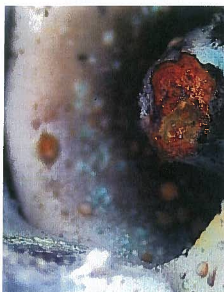
(PHOTO 5) —Microscopic view of the end of a contact of a 500 watt fixture showing arc by-products.
