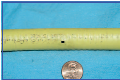
Figure 8: Photo of perforated CSST without pyrolysis.
