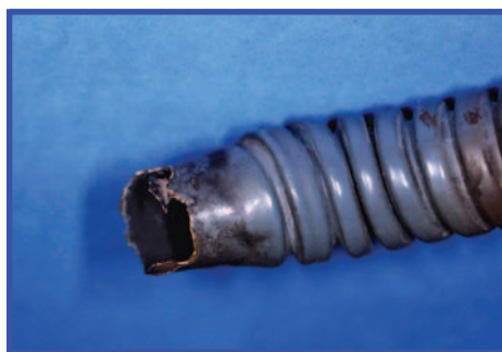
Figures 10a & 10b: Bottom and side respective views of failed gas line from appliance connectors (Not CSST).
