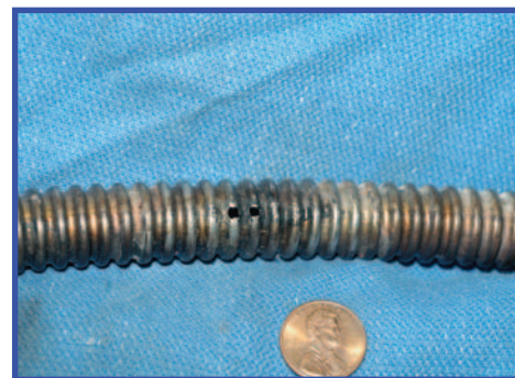
Figure 11: Adjacent perforations in CSST.
